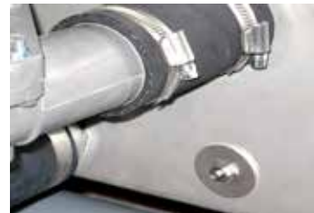
Detergent dispensing system. The dishwasher has the necessary fittings for a detergent and drying agent dispenser.
