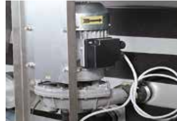
Self-emptying pumps in the washing and rinsing zones improve hygiene levels.
