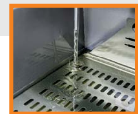
Filtered oil is pumped back into the fryer
