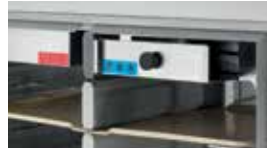
Drawer for enhanced cooling with CO2 pellets during transportation.
